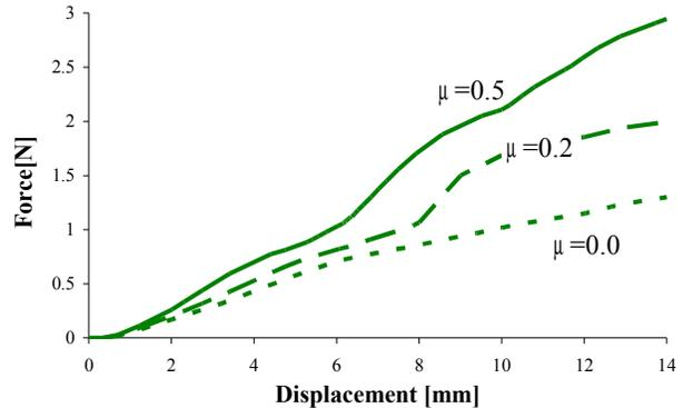
Figure 5 Sequence of contour plots during the in-silico clam shell test and plot of force versus displacement showing the influence of friction on the simulation results.
