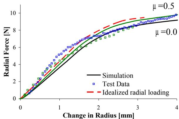
Figure 9 Photograph of the segmental compression test using device manufactured by Machine Solutions Inc. (MSI) Radial Force Gauge RX500 and comparison of segmental compression in-vitro and in-silico test results. Also shown are the results for the idealized radial loading.
