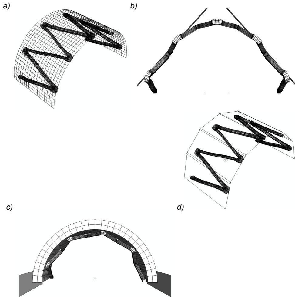
*Figure 2. FEA models of the a) loop strap; b) clam shell; c) flat plate crush ; and d) segmental compression tests*
